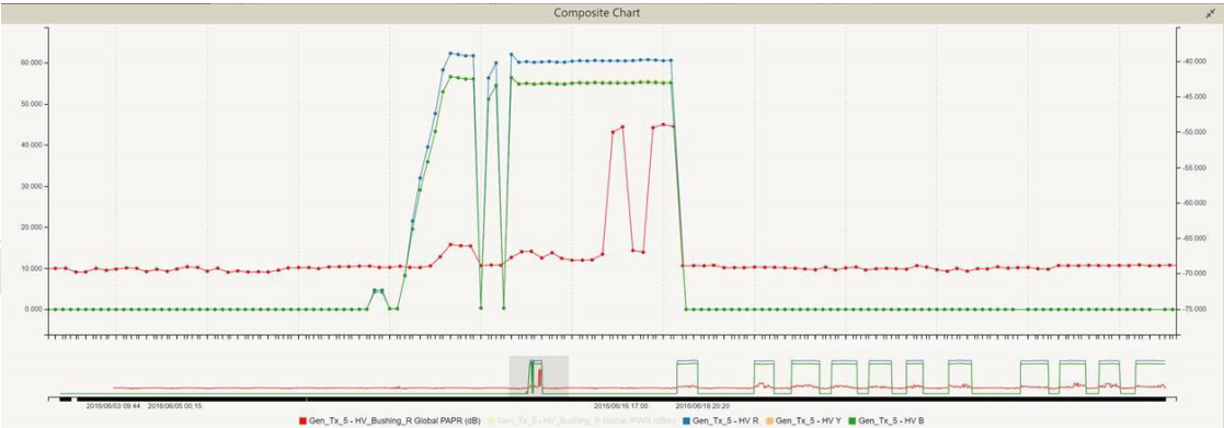
ANALYZE DATA FROM VARIOUS MODULES PD from a bushing overlaid by leakage current provides more context for analysis
