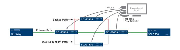
Deploy software-defined networks to take advantage of the ability to engineer network traffic with predetermined primary and backup paths that fail over in less than 100  $\mu$ s when any link is lost.
