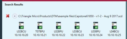
Multiple IEDs in a substation can be browsed to easily find the data you need. Available IEDs can be scanned by IP address range or using configuration from SCL files.
