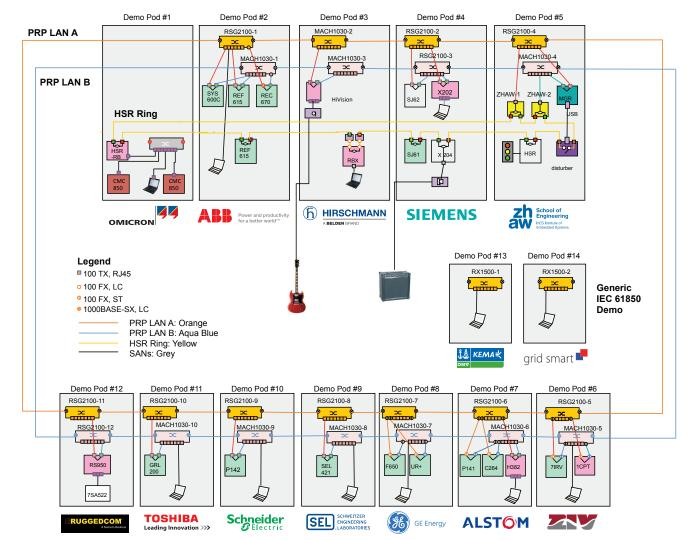
Fig 2. Network Topology of PRP/HSR Interoperability Demonstration and Generic IEC 61850 Demonstration at UCAlug CIGRÉ 2012 Booth
